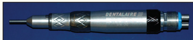
DA700A – Low Speed, Light Weight, Lube Free Handpiece (5000 RPM)
